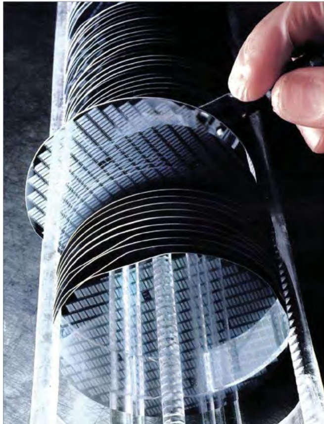
Fig. 10 —Semiconductor production at Fairchild Camera and Instrument Corporation that was a part of Schlumberger from 1979 to 1987. Silicon wafers in process at the Fairchild South San Jose plant, California, in 1980. Each wafer contained several hundred large-scale integrated circuit chips (courtesy of Schlumberger).
