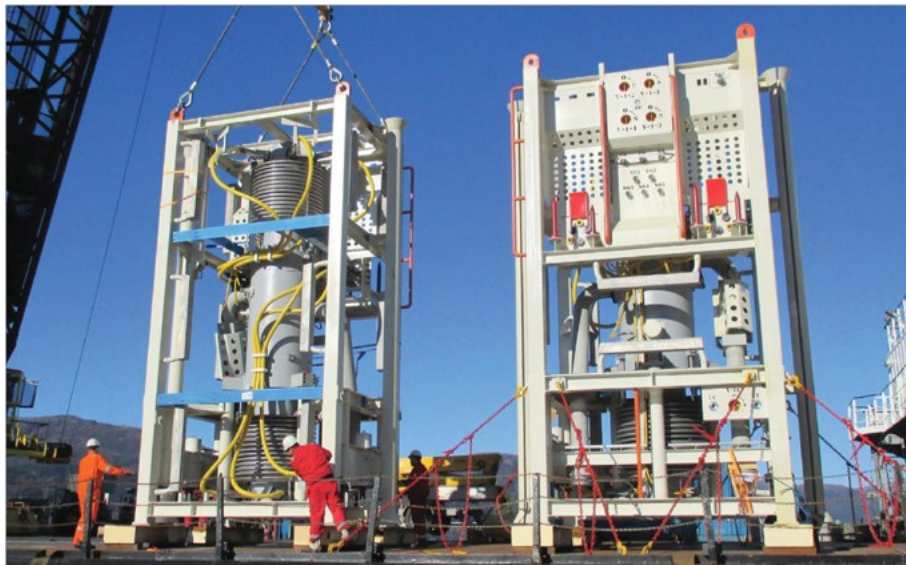
Fig. 20—Two Multiphase Compressor units at the OneSubsea facility in Horsøy, Norway (courtesy of Schlumberger).
