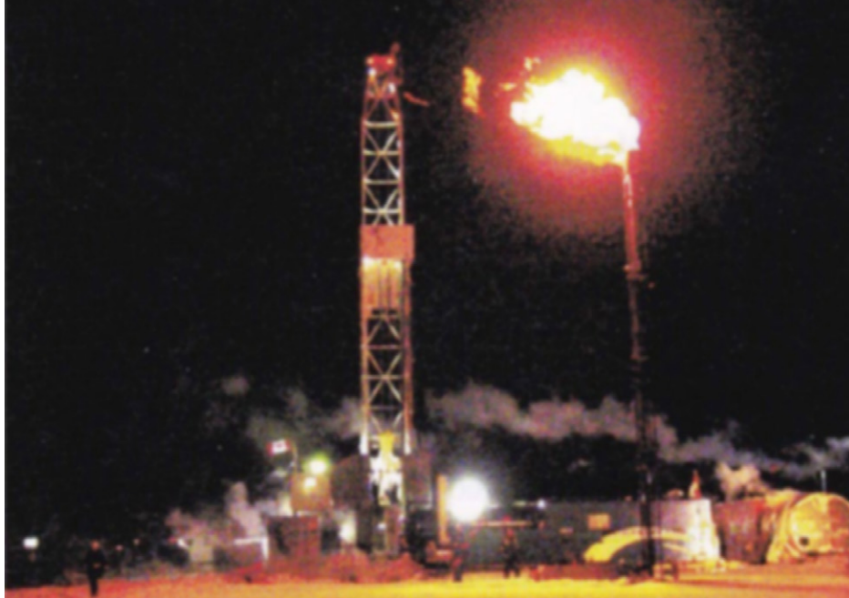
Fig. 2 —Photo of the gas flare from the thermal production test in the Mallik 5L-38 research well (courtesy of the Mallik 2002 Gas Hydrate Production Research Well Program).
