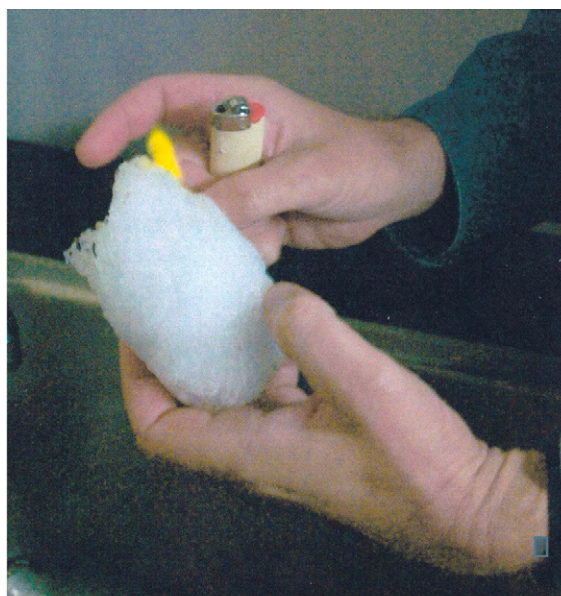
Fig. 1 —Photo of a gas-hydrate-bearing core from the Mallik 5L-38 research well. The gas hydrate is the white material that has been ignited by the lighter in the technician's hand (courtesy of the Mallik 2002 Gas Hydrate Production Research Well Program).
